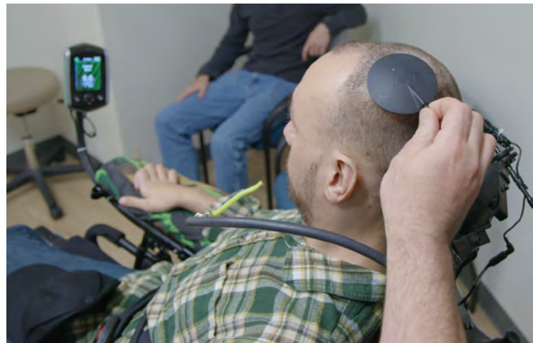
Left: The coin-sized Neuralink implant contains a small battery, advanced low-power chips and 64 threads containing 1024 electrodes. Right: A wireless charger is used to recharge the implant battery.
