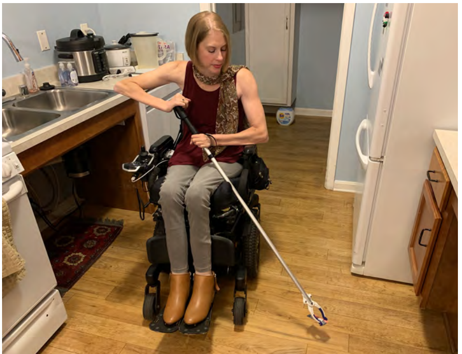
The Grip-Free Grabber was designed for people with limited hand function to be able to pick small items off the floor or from up high.
